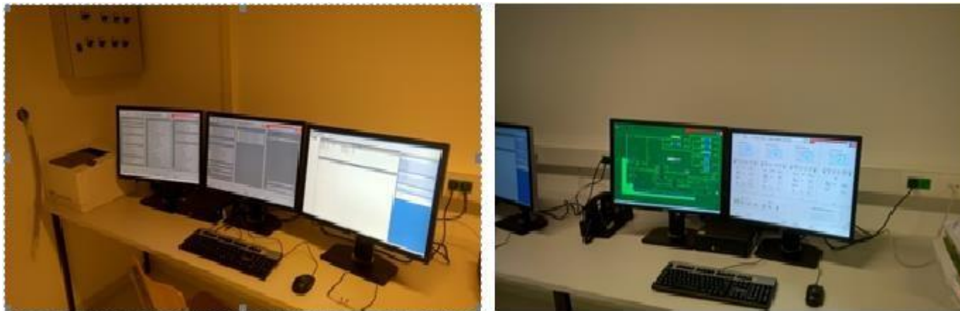
Figure 11. Instructor's and student's station of the KONGSBERG simulator
