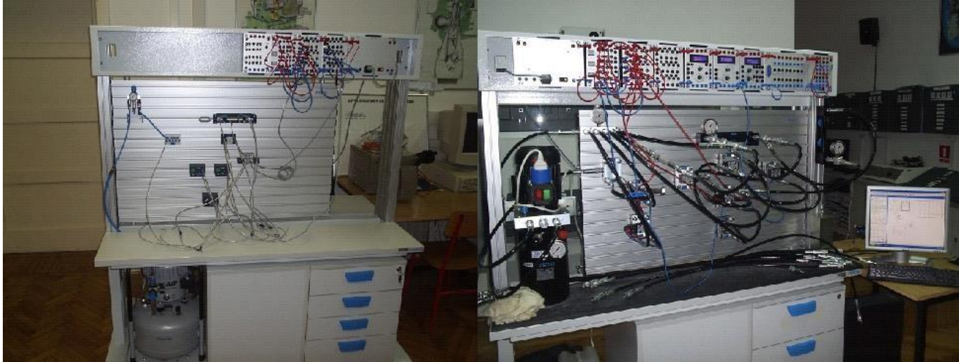
Figure 15. Didactic desk for pneumatics and electro pneumatics & Didactic desk for hydraulics and electrohydraulic ➤
