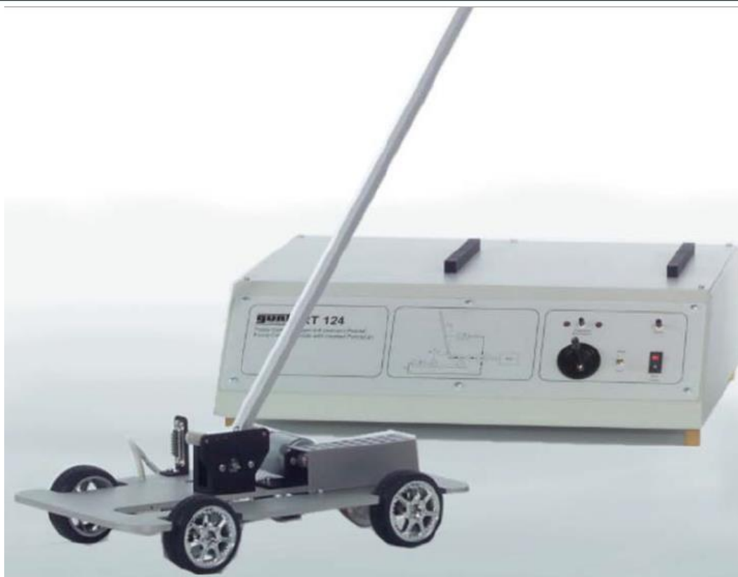
Figure 23. GUNT RT 124, vehicle with inverted pendulum, hardware simulator and software for fuzzy control
