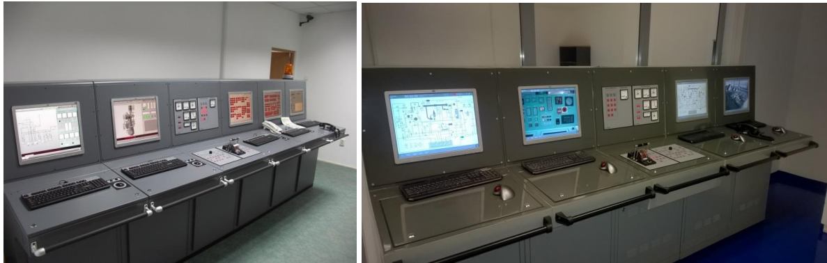
Full Mission Engine Room Simulator (Transas ERS 5000) connected (integrated) with Main bridge (Transas NTPRO 5000)
