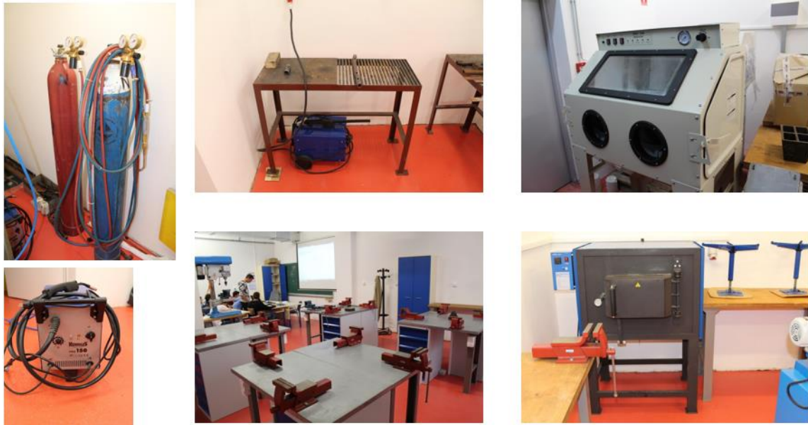
Hand tools and welding cabinet, sanding and heat treatment equipment
