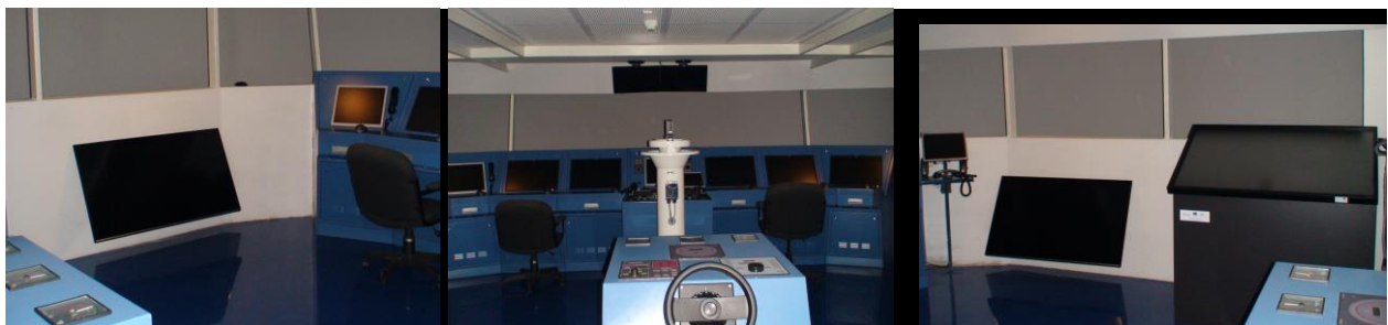
Main FMB 1 with DP Class 2 , Manoeuvring station + Real Pelorus Stand (Class A NAV)
