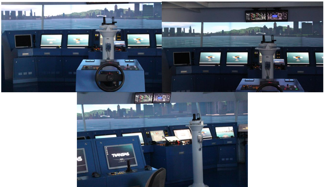
Main FMB 1 with DP Class 2 , Manoeuvring station + Real Pelorus Stand (Class A NAV)
