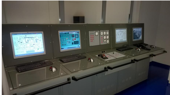
Full Mission Engine Room Simulator (Transas ERS 5000) connected (integrated) with Main bridge (Transas NTPRO 5000)
